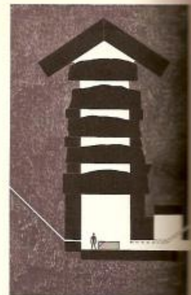
THE KING'S CHAMBER was roofed with enormous granite slabs that formed five weight-relieving compartments. Now, though many slabs have cracked, the roofing remains in place.
